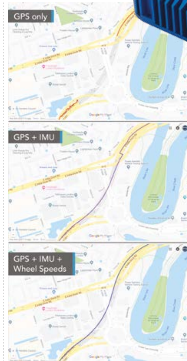
ABOVE: IMU and wheel speed data retains centimeter-level positional accuracy for up to five minutes in environments with no clear view to the sky
