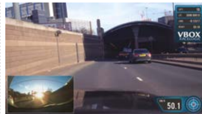
ABOVE: Multifrequency GNSS retains 2cm positional accuracy even in built-up urban areas
