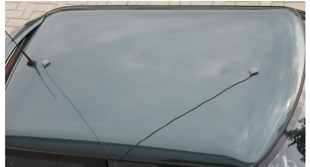
Figure 2: Twin antenna configuration
