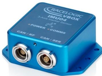
For accurate testing, even in areas where the view of the sky is obstructed, VBOX 3i can gather additional information from an IMU (Inertial Measurement Unit – pictured left) and combine this with the GPS data in real-time to improve the quality of the parameters measured.
