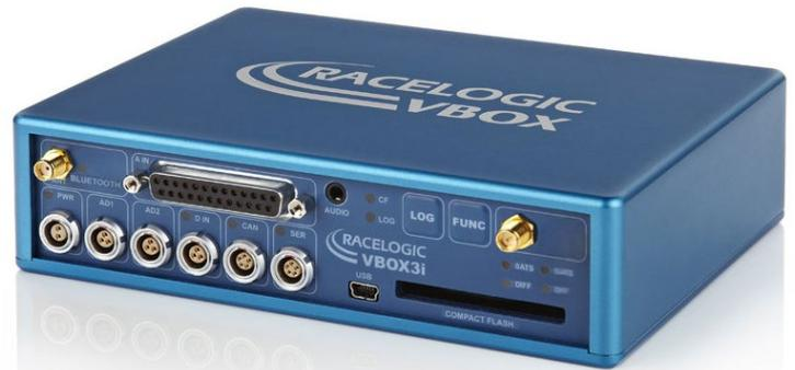
VBOX 3i comes in three versions: Single Antenna, Dual Antenna and RTK. When used with a DGPS Base Station, VBOX 3i Single Antenna can achieve 50 cm positional accuracy. (An RTK enabled version of the VBOX 3i can obtain <2 cm positional accuracy in conjunction with an RTK Differential Base Station.) This enables users to measure parameters within acceleration, deceleration, braking, ABS and ESP testing, handling manoeuvres and many other types of high dynamic testing.
